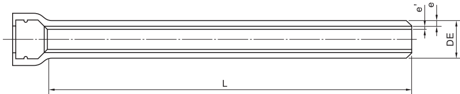
Dimensions of pipes thickness
